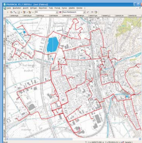
Smallworld's GIS data model forms the basis for the network calculation program (here: PSS/SINICAL).
