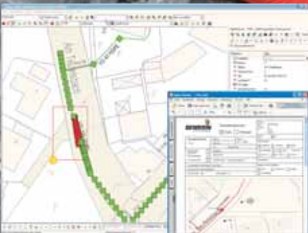
With SeCuRi SAT you can provide a preliminary damage drawing onsite. Damage found is documented, classified and is handed over to the reporting system and/or to maintenance planning.
