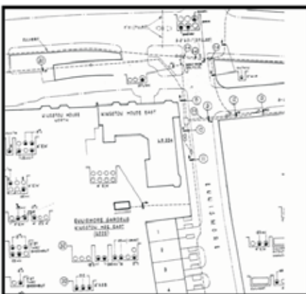
What you see is what you get: The representation shown on the raster is recreated in vector. The single lines contain detailed attribute data of the cables inside the tray.
