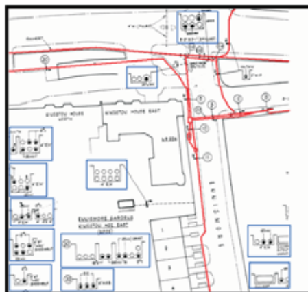
What you see is what you get: The representation shown on the raster is recreated in vector. The single lines contain detailed attribute data of the cables inside the tray.
